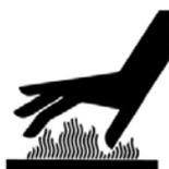
Pumps operated in these circumstances may experience a build up of vapor pressure and may contain scalding hot water. Opening the pump may cause serious personal injury. In order to avoid the possibility of personal injury, make sure the suction and discharge valves are open and strainer pot temperature is cool to touch, then open with extreme caution.
