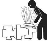
**HAZARDOUS PRESSURE: STAND CLEAR OF PUMP AND FILTER DURING START-UP**
